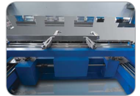
Four (4) axes Back Gauge, X-R-Z1-Z2
