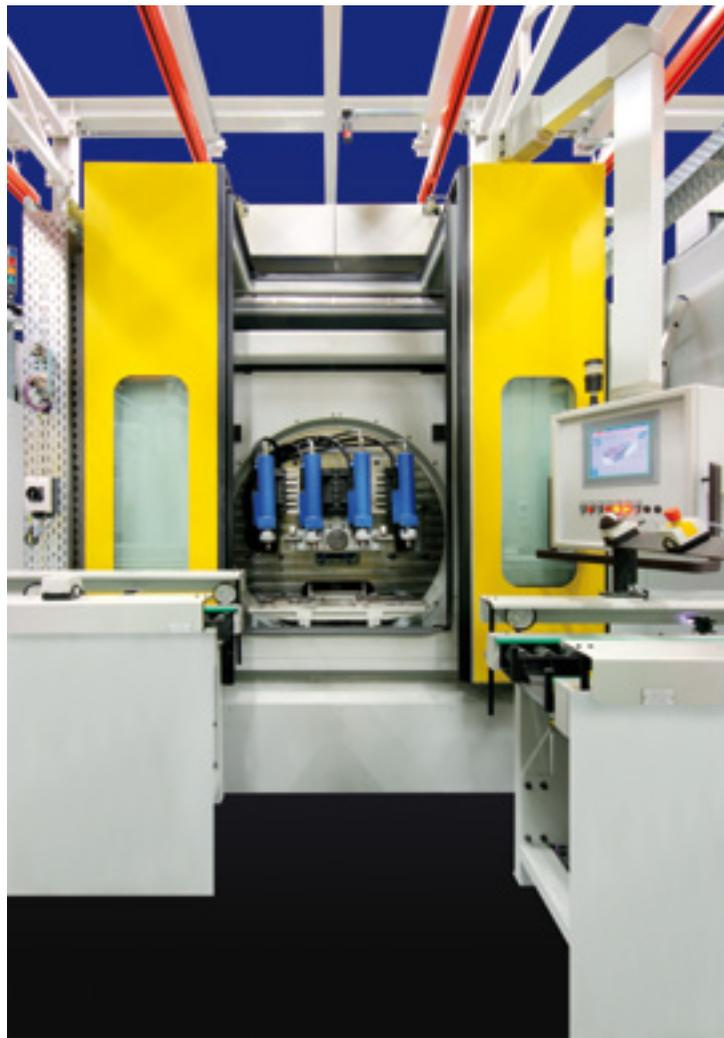
*Sand Removal - Decoring Systems \ Mössner systems use electric and hydraulic hammering and vibration, as well as rotating components to thoroughly remove sand from castings.*
