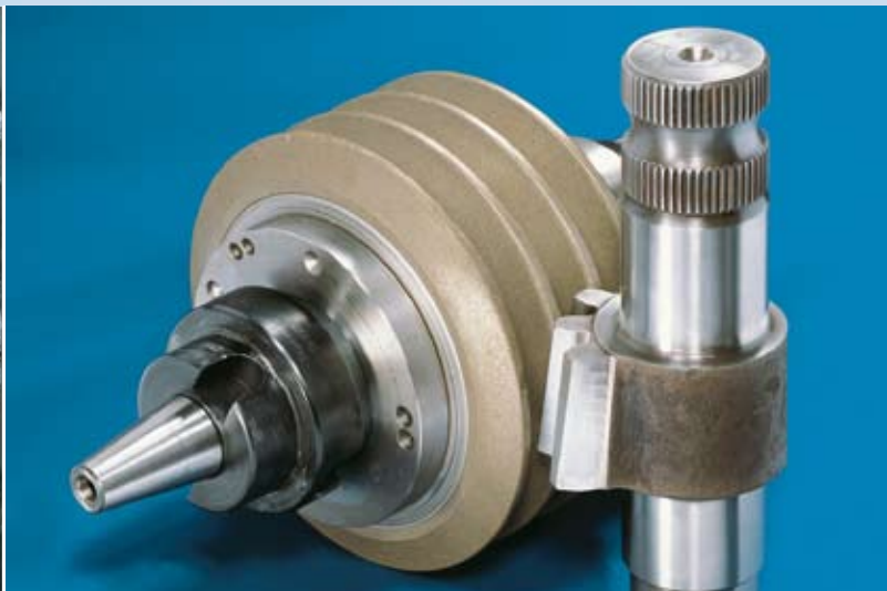
Special application CBN grinding of a steering segment
