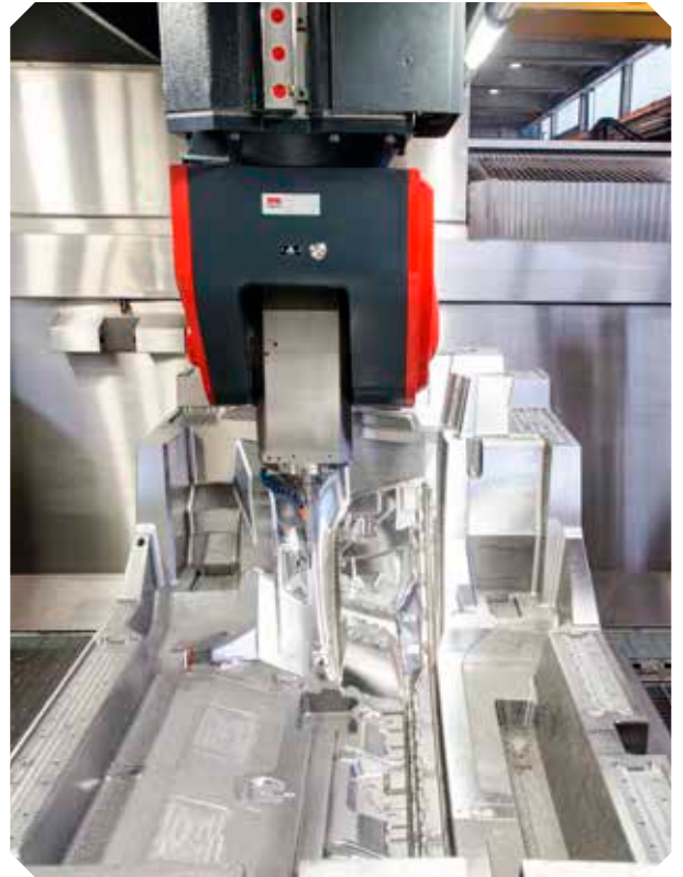
Machining of a mold for automotive industry
