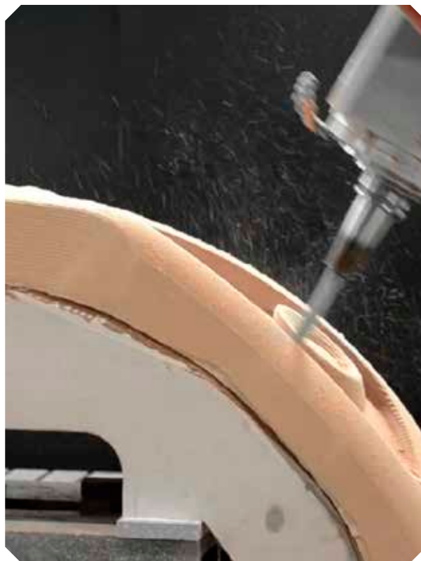
Machining of a resin model
