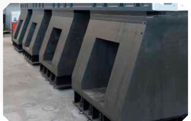
Epoxy Concrete Columns
