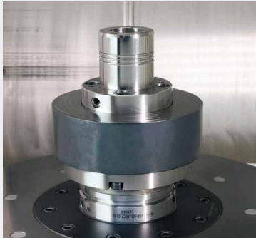
Workpiece clamped by hydraulic expansion toolholder
