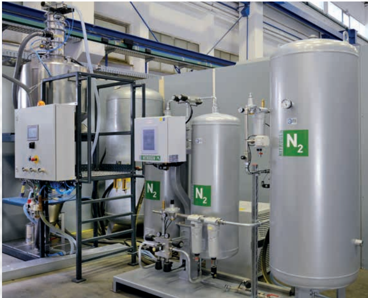
Nitrogen generator The nitrogen generator permits the creation of the inert gas atmosphere with a nitrogen purity of up to 99.9 %.
