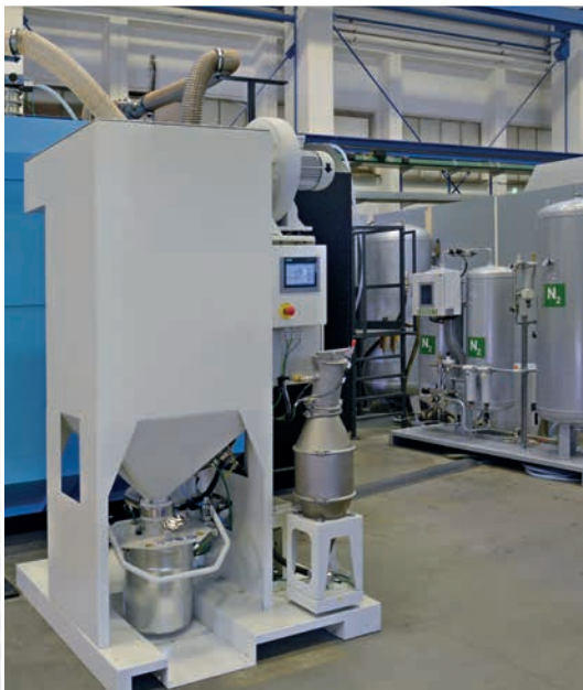
Extraction system Fume extraction system (filtration) with a sinter-plate filter in combination with safe passivation and integration into the inert gas circulation system.
