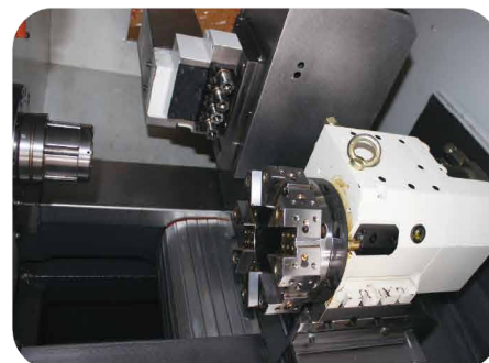
➤ Hydraulic Turret + Cross Drilling Device
