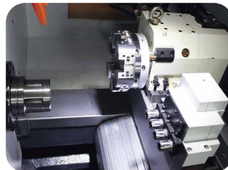
➤ Hydraulic Turret + Face Drilling Device
