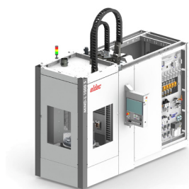
MIND-L 1000 S: Induction hardening machine for large quantities with maximum and consistent precision
