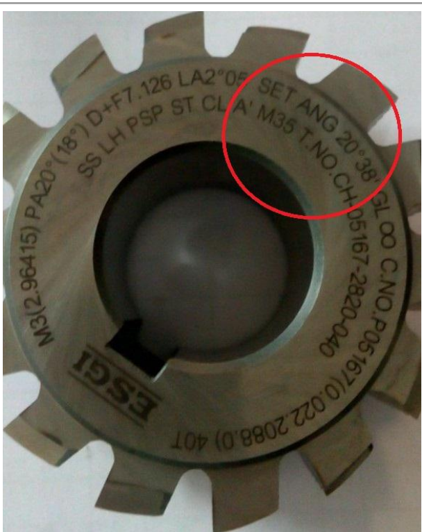
Picture 4 (Marking on Hob for Helical Gear)
