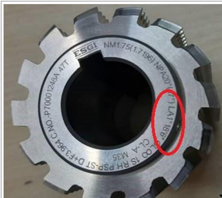
Picture 3 (Marking on Hob for Spur Gear)
