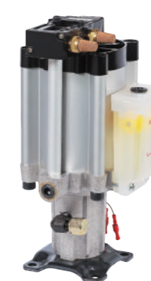
▲ Pneumatic/hydraulic converter (8 times) · Air pressure source 6kg/cm 2 · Solenoid valve DC24V or AC110 / 220V
