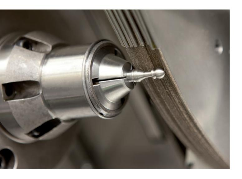
The GRINDSTAR machine concept replaces turning through the use of dressing-free high-speed plunge-cut grinding. This can open up enormous potential for savings, in particular when working with large production volumes.
