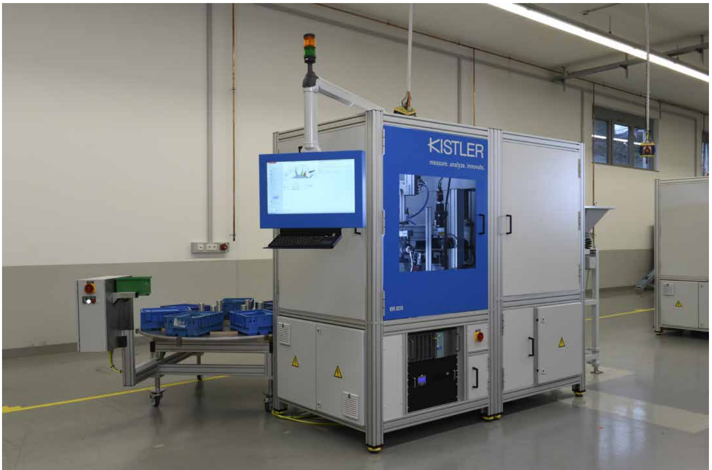
Flexible structure – inside and outside: thanks to its modular design, the KVC 821 automatic testing and sorting system can be equipped and extended for each specific application.
