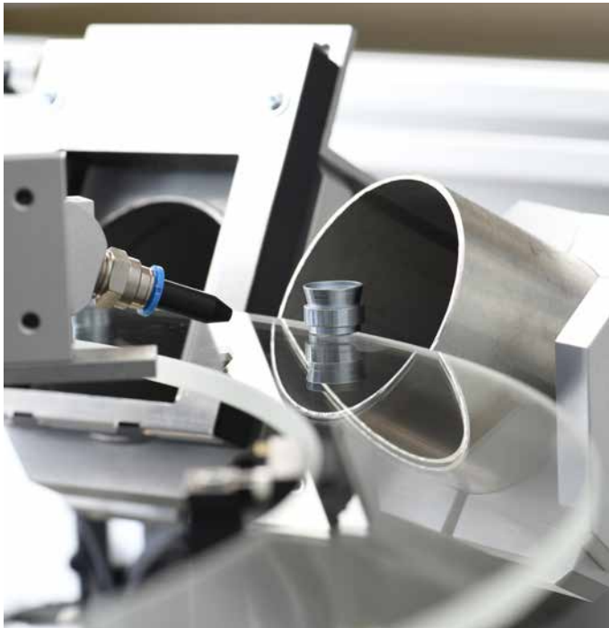
Exclusion and ejection control for bad and good parts upstream of each station
