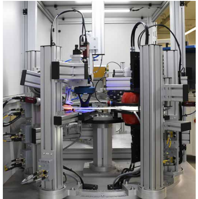
Test chamber with rotary plate and various testing stations
