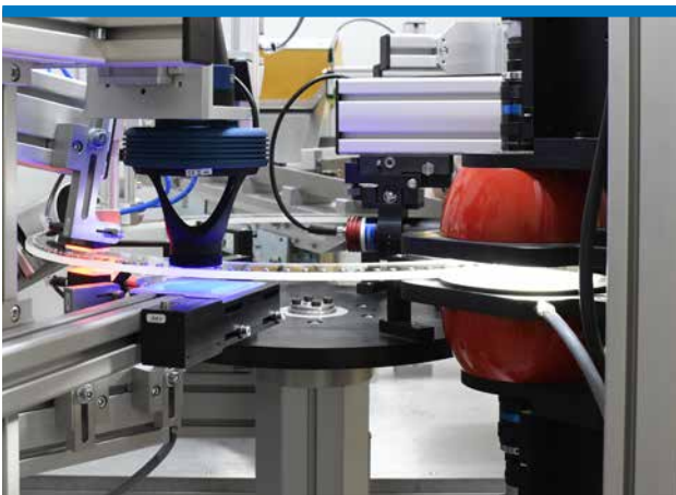
All variants of illumination with reflected or transmitted light can be implemented in the KVC 821.
