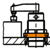
with threaded flange and grooved nut
