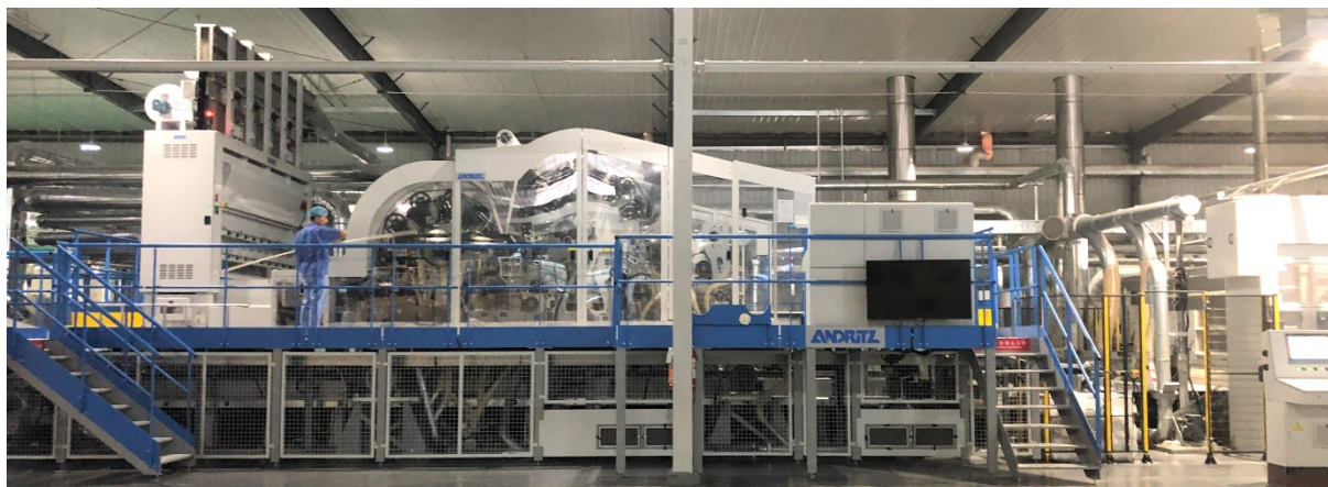
High-speed TT card combined with the JetlaceEssentiel hydroentanglement unit in operation at Kingsafe
